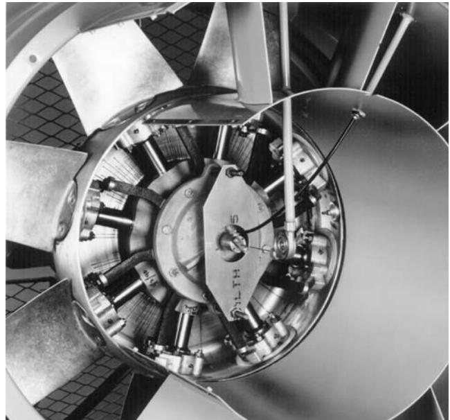
A close-up of the pneumatic controllable pitch impeller mechanism viewed through the standard access panel. Pneumatic supply air (80 to 100 psi) is introduced to the diaphragm through the rotary union (center of photo with feedback cable attached) inflating the pneumatic piston forcing the spider arms to move away from the hub and increase the blade angle of attack.
