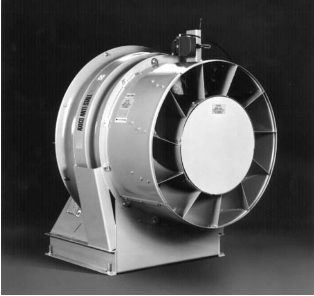
View of AXICO ANTI-STALL® fan from discharge. Honeywell industrial-gauge pilot positioner with closed-loop feedback cable is shown standardly mounted on top of straightening vane section. Bolt-on vane section allows 360° rotation to allow simple field adjustment for improved job site accessibility of pilot positioner.
